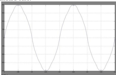
Figure 4 Current Waveform Before Filtering
